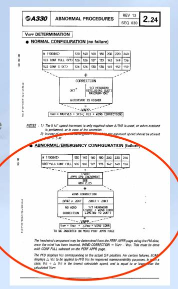
Determine V<sub>REF</sub> (= V<sub>LS</sub> CONF FULL) on the table for expected landing weight.
